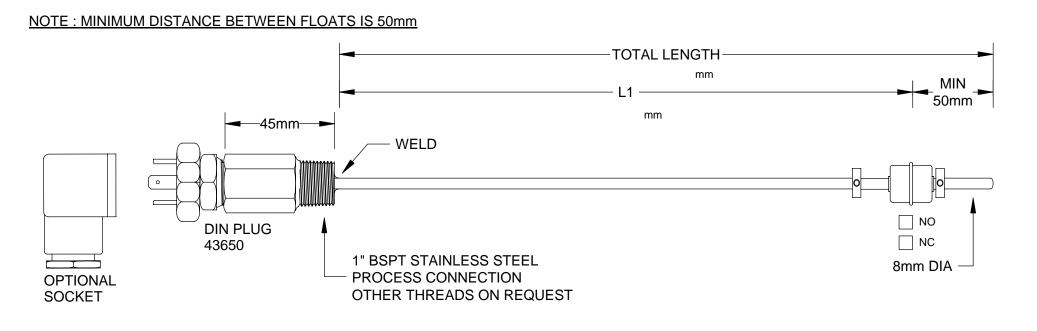
STANDARD - NO or NC CONTACT RATED AT 32V AC/DC @ 500mA RESISTIVE LOAD
